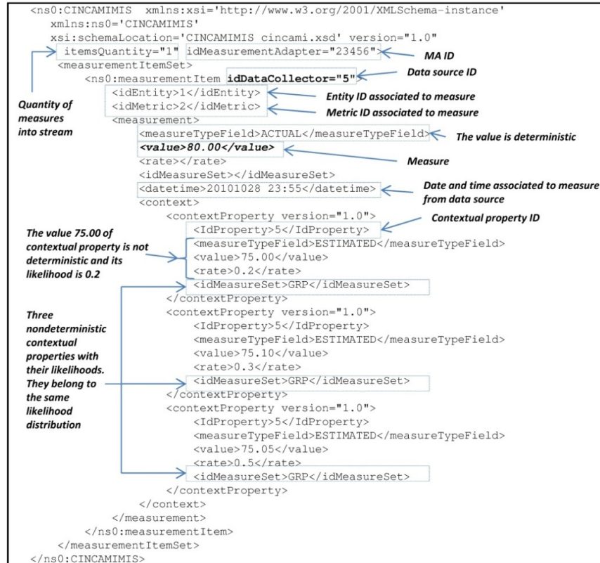
Fig. 3. Annotated XML schema of a C-INCAMI/MIS stream.
