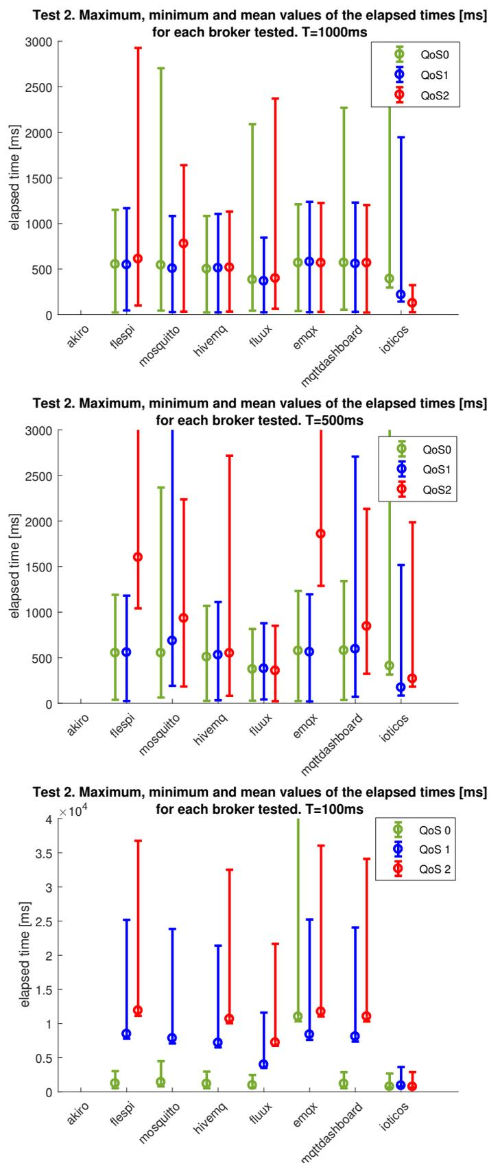
Fig. 8: Minimum, mean and maximum elapsed times of the messages published in the second test with transmission intervals of 1000ms (top), 500ms (middle) and 100ms (bottom) for each QoS tested
