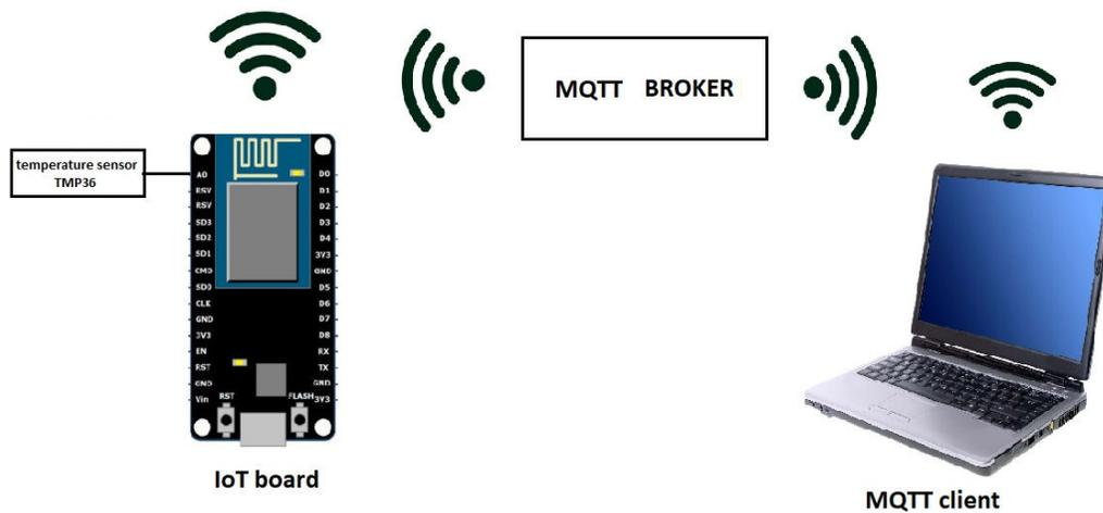
Fig. 5: System layout in the first and second tests
